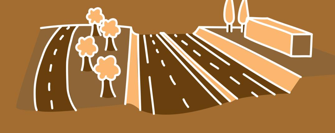
Natural protection induced by the highway geometry, built below natural ground level.
